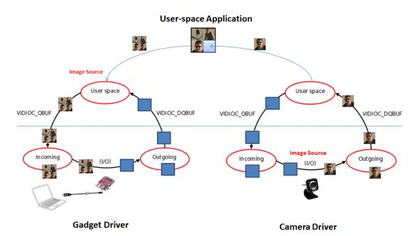
Once setup process is finished and streaming I/O starts, the systems goes into an infinite loop illustrated in the following diagram:
